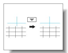
9 If the lines are shifted as shown at the right, touch to specify the desired positive adjustment for "X" (between +1 dot and +6 dots).
